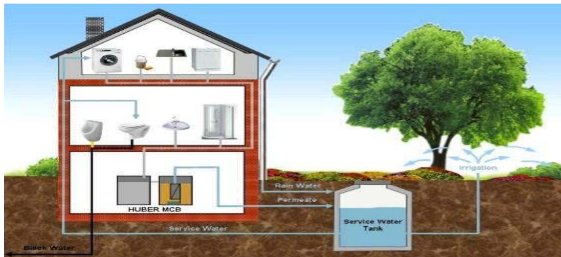
Figure 10: Grey Water Collection & Recycle Process
